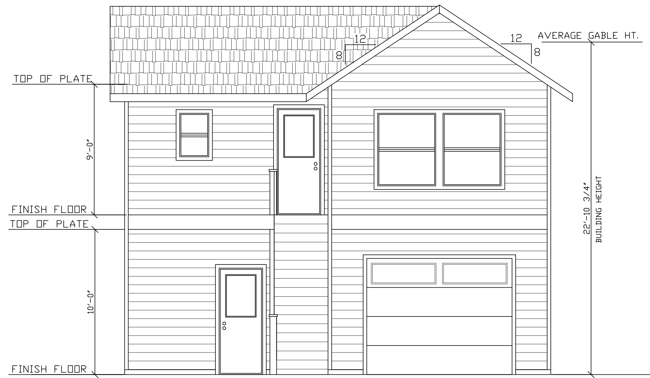
FRONT ELEVATION SCALE: 1/4" = 1'-0"
